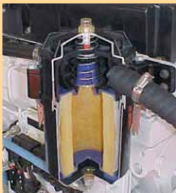
Cummins QSM11 marine engine with CCV cutaway
